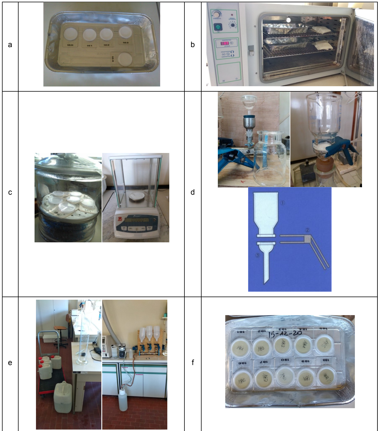
Fig. 2 - (a) Membrane filters before first drying; (b) filters during the first heat treatment in the oven; (c) filters in the dryer and analytical balance; (d) assembly of the filtration system; (e) measurement of the sampling volume and filtration; (f) filters after the filtration (the deposit of the suspended material collected is evident), ready for the second heat treatment and, in the end, weighing.
