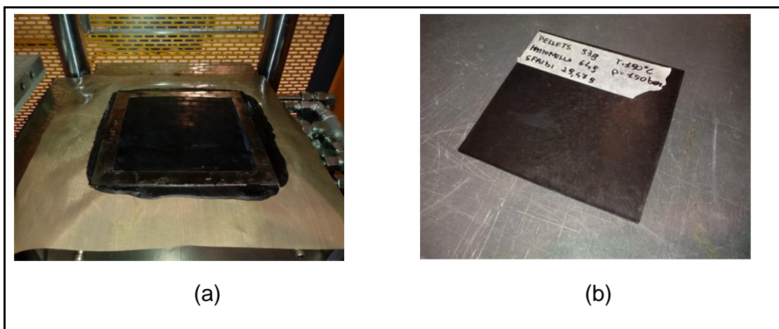
Figure 6 : Moulded composite materials before (a) and after (b) sprue removal.
