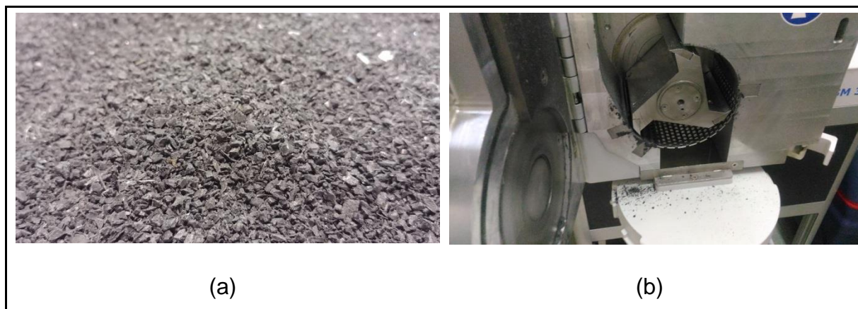
Figure 2: milled samples (a) and details of the cutting mill after milling (b).
