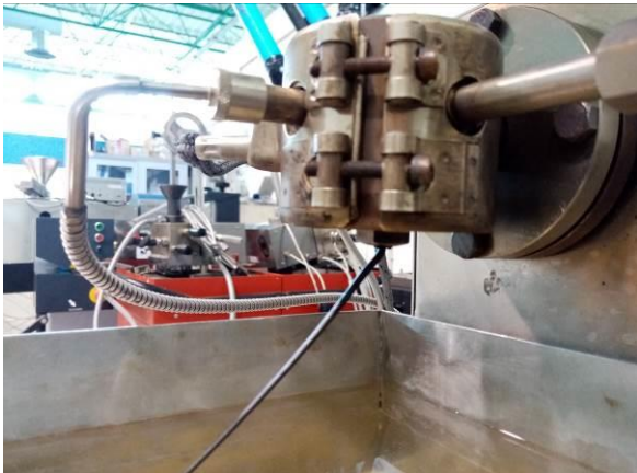
Figure 14: Extrusion process for the production of vPA6/rCF pellets.
