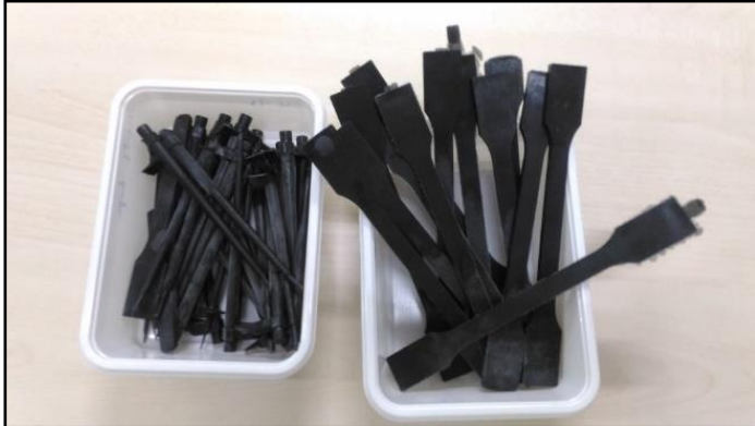
Figure 7: Dog-bone samples and sprues in PP/rCF (10 wt.%) 3mm_US.
