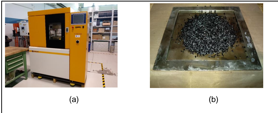
Figure 5 :COLLIN P 300 P/M platen press (a) and materials charged into a squared mold (b).
