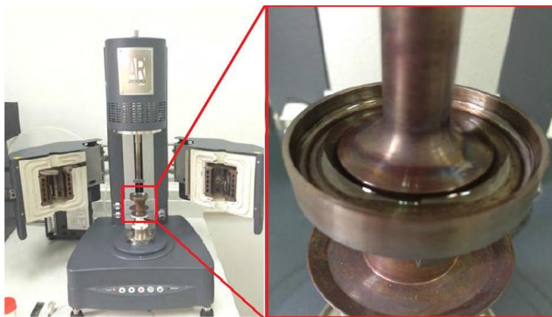
Figure 12 AR2000 ex rheometric system used and sample positioning for viscosity measurements.
