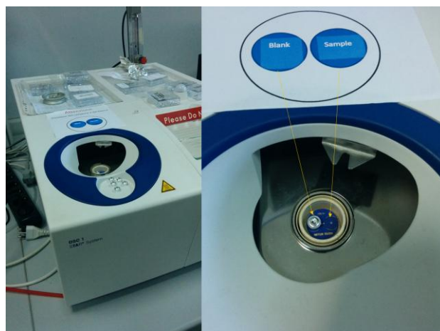
Figure 11 used instrument, TGA/DSC Mettler Toledo module.
