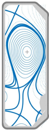
Figure 10. Example of a Jellyfish poloidal configuration with three X-points in the lower divertor region. LFS parallel connection length peaks \sim 120 \text{ m} . A strong reduction in peak heat flux compared to the reference single-null reference configuration. Adapted from [63]. CC BY 4.0.
