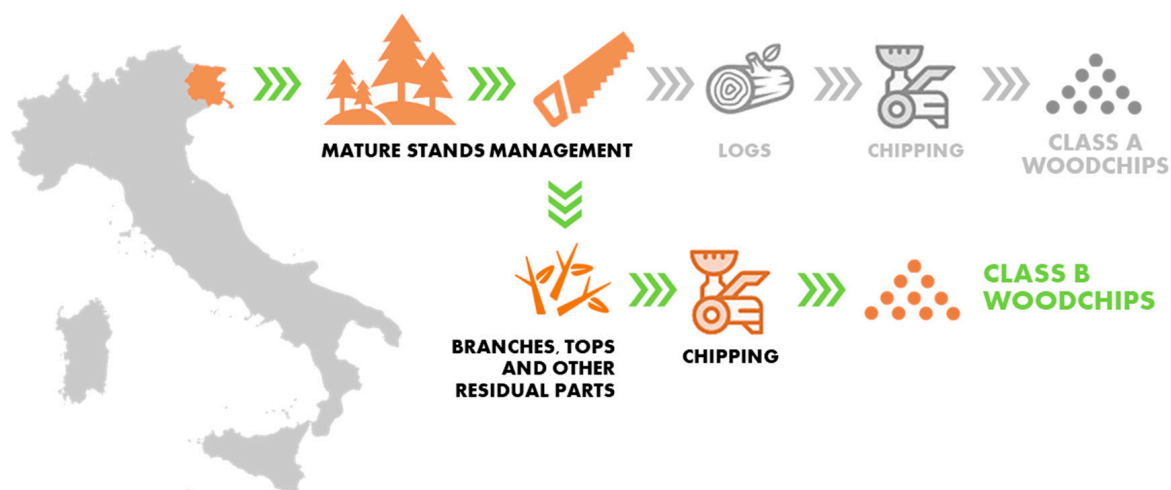
Figure 1. Case study for the production of the forest woodchips (colored icons and arrows identify the reference production chain).
