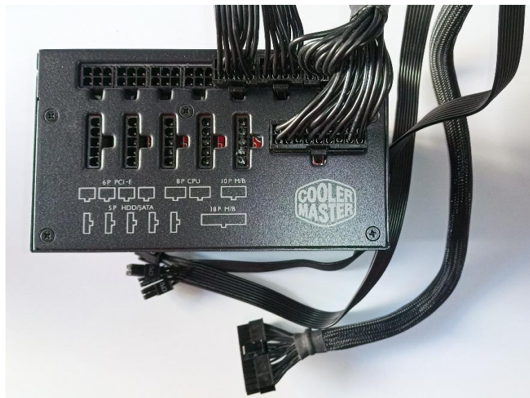
Fig. 7: Regular power supply unit, with several connectors for additional power lines.
