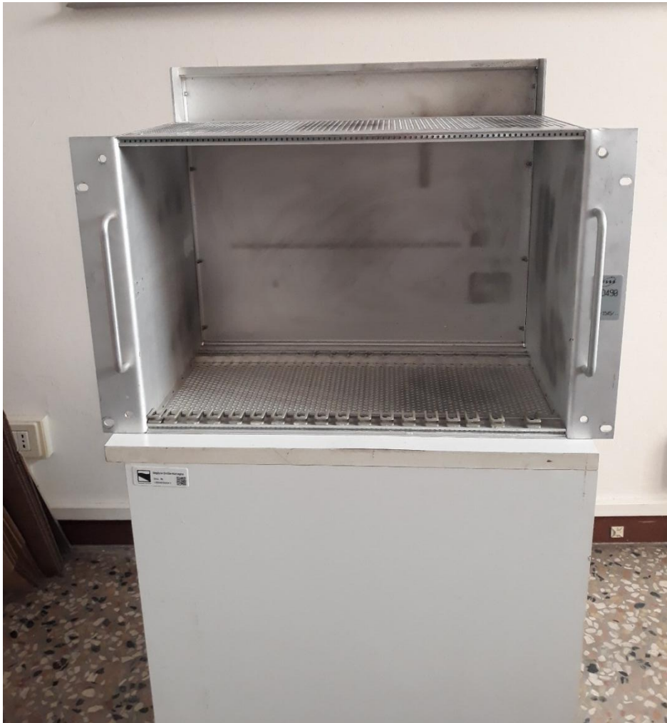
Fig. 2: Metal enclosure with plastic rails on the internal bottom and top (hidden).
