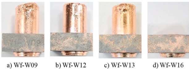
Fig. 9. Wf/W-Cu blocks after OFE-Cu casting.
