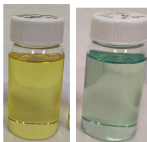
Figure 8. HCl fractions containing Fe (left) and Ni (right) after chemical separation.
