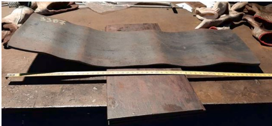
Fig. 1. Waved shape of the heavily cold worked plate (alloy 3387).
