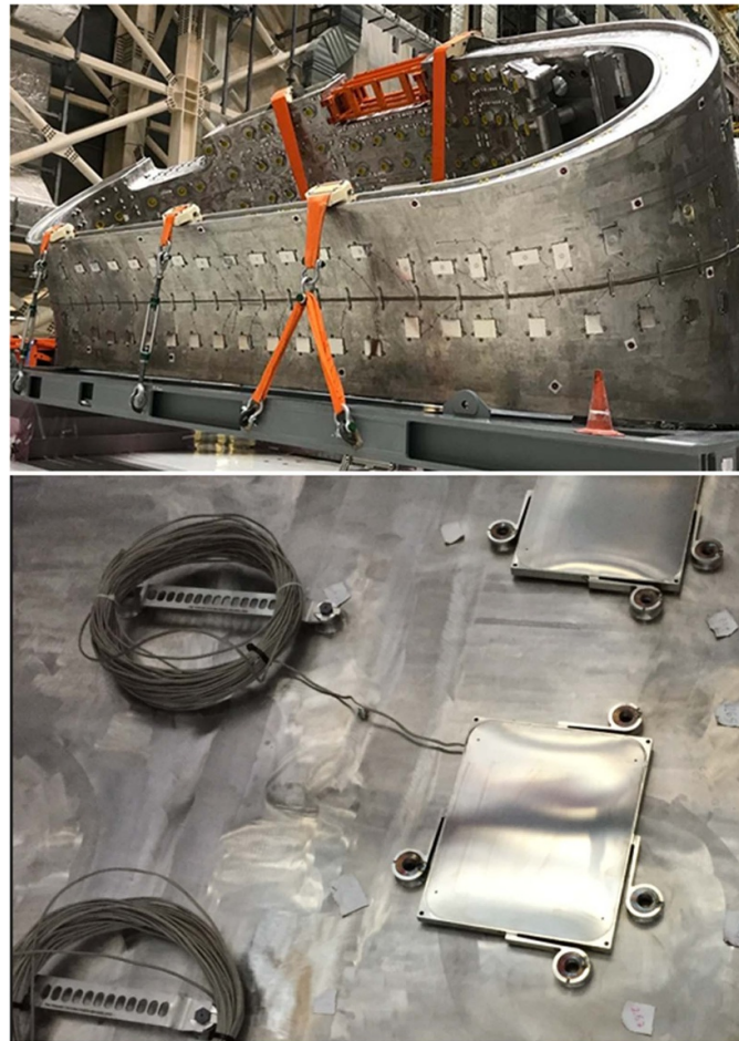
Figure 8. Top: ITER VV Sector 6, the inboard outer vessel pickup coils tangential (top row) and normal (bottom row) clearly visible. Bottom: Close-up of a tangential coil. Inconel plates and fiberglass preload the winding pack into the Inconel case; Four welds to vacuum vessel bosses hold the sprung legs in place to allow an operating range 70–573 K without rotation.
