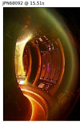
Figure 90. Interior of JET illuminated by its plasma emission, contaminated following a sodium influx. The yellow color shows that post-pulse analysis may not always be necessary. The complex interior surfaces and the sharp outline of the last closed flux surface can be seen.
