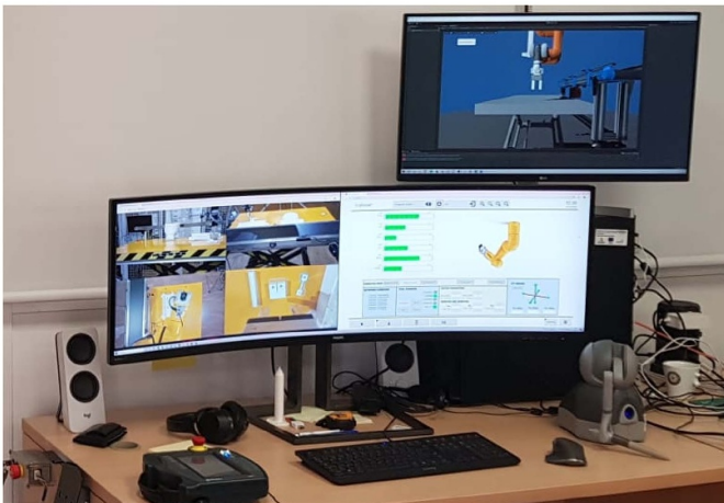
Figure 36. Operator Workstation without direct view to the robotic cell. Image Courtesy of Francisco Barranco (UGR-ES) and Elio Valenzuela (PHD student at UGR-ES).
