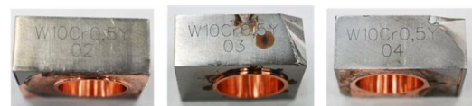
Fig. 6. Blocks #Y_02, #Y_03 and #Y_04 after OFHC-Cu casting and bore hole machined to 15.06 mm.
