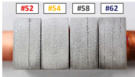
Fig. 18. Mock-up ENEA 80 after HHF test in GLADIS facility (20 MW/m 2 , 1500 pulses, 10 s pulse, cooling water T_{in} = 130 °C, flow rate 1.6 l/s).
