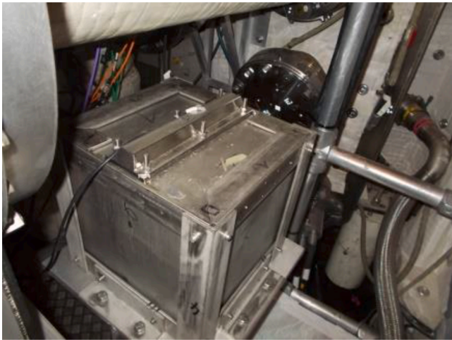
Fig. 12. Photo of the HCPB TBM mock-up installed close to the front collimator of the beamline in Octant 8. The dimensions of the HCPB TBM mock-up are 30 \times 29 \times 31 \text{ cm}^3 . The stainless steel box is filled with beryllium and it contains two steel double cassettes filled with \text{Li}_2\text{CO}_3 powder [38].
