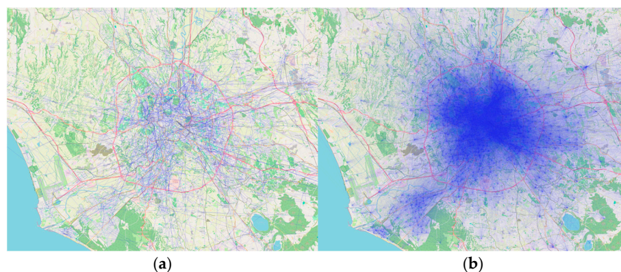
Figure 4. Origin–destination trips generated from FCD (a) and synthetic (b) samples during the weekday morning peak hour (3 October 2022, 07:00–08:00) across the province of Rome. The synthetic dataset corresponds to a simulated fleet of 1.5 million vehicles (OpenStreetMap contributors, https://www.openstreetmap.org , accessed on 27 November 2025).
