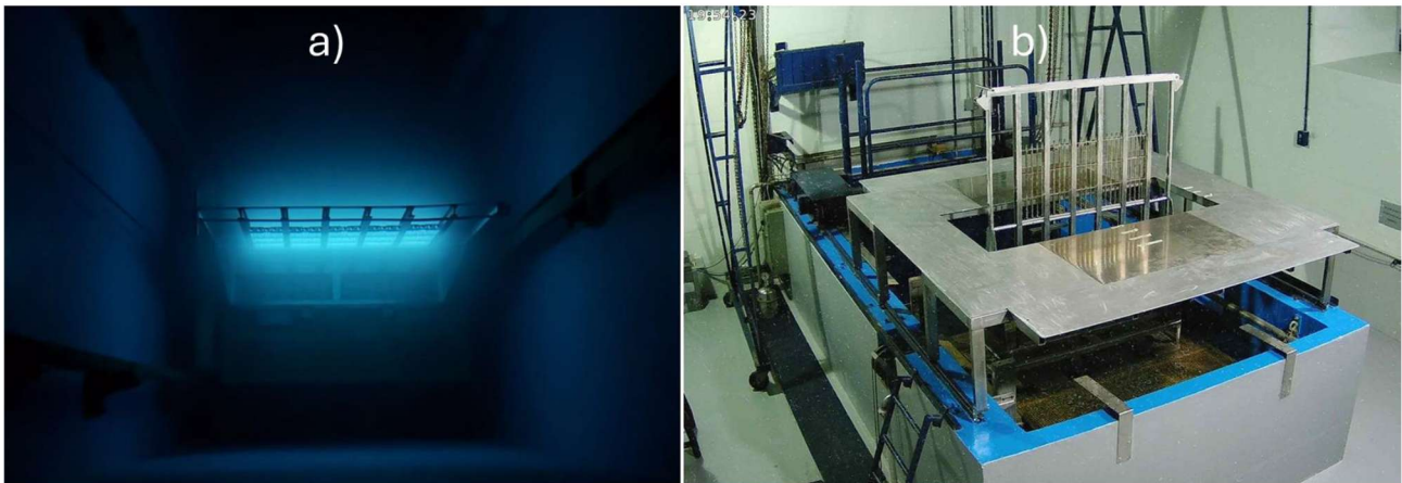
Figure 4. Calliope source rack at the bottom of the storage pool and b) source rack within the irradiation cell (picture acquired by remote camera).
