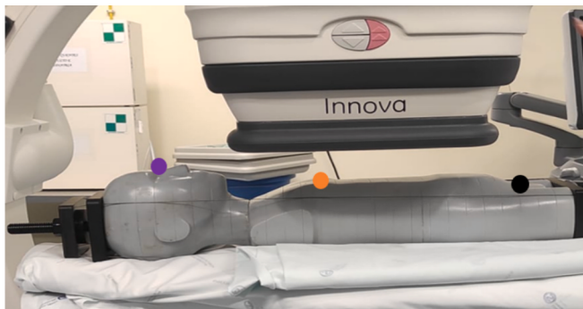
Fig. 5. CIRS ATOM 705. Dosimeter positioning: Purple dot nose, orange dot heart and black dot gonads. (For interpretation of the references to colour in this figure legend, the reader is referred to the web version of this article.)
