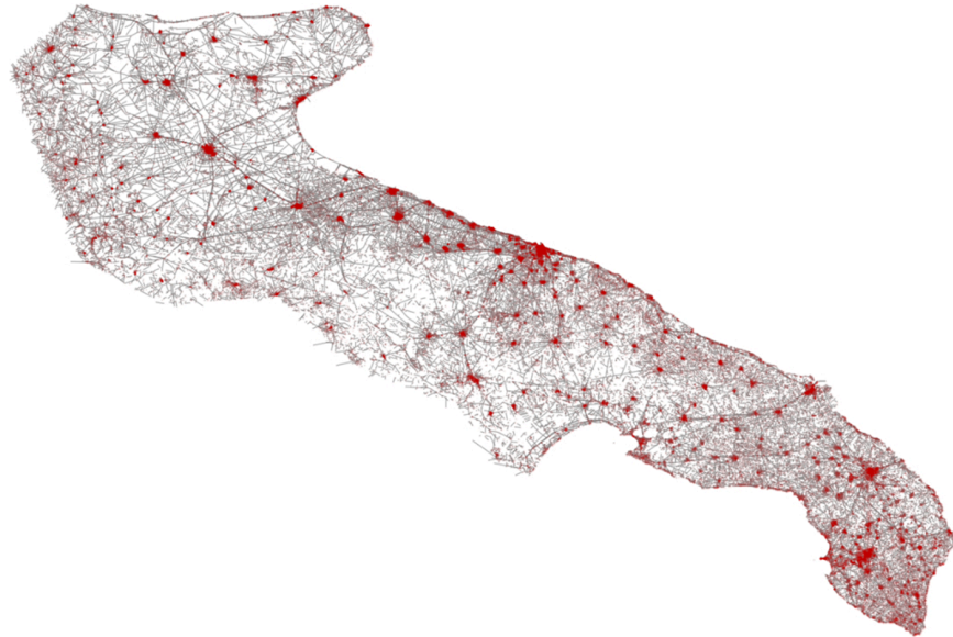
Fig 10. Graph representation of the Apulian road network illustrating nodes as road LineString endpoints and links as roads. The map is generated using the Folium open source library, which uses OpenStreetMap as a map source [50].
