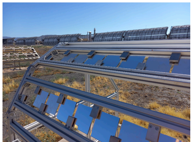
Fig. 2. Sample exposure rack with marked positions and sample numbers during main and extra campaign (left), detailed view of first inclination rows from the horizontal, with sample holders (right).
