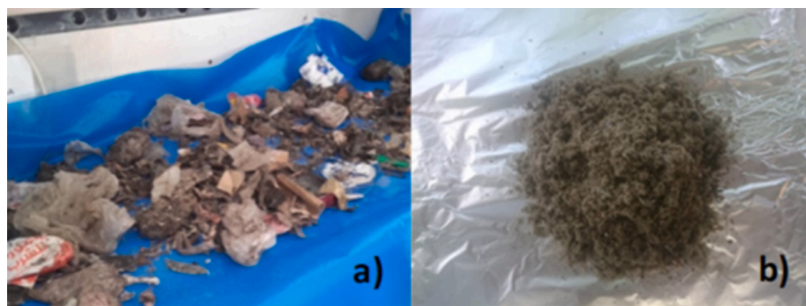
Fig. 6. a) The municipal solid waste (as received); b) Milled MSW inert free.
