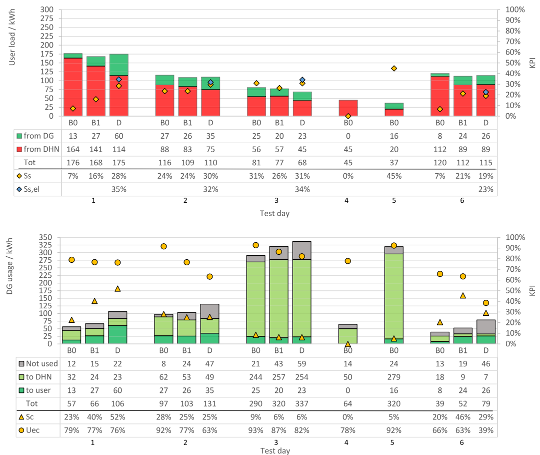
Fig. 8. User load sharing between DHN and DG, distribution of DG energy production, and KPIs for the representative days. Case studies B0-B1-D.
