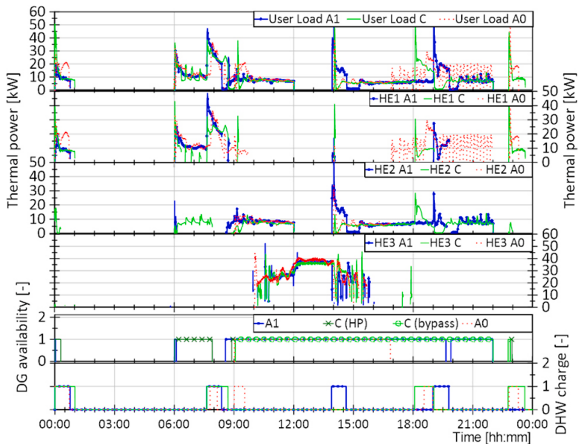
Fig. 11. Day 3. Interaction between the HEs according to thermal demand and DG availability. Case studies A0-A1-C, DHN supply and return 80/50 °C
