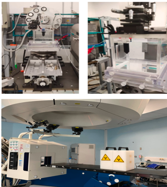
Fig. 2. Representative photos of the experimental setups for IR eye exposures Top: two different views of the setup for X-ray exposures in the INMRI ENEA premises, with the darkened Falcon tube positioned with its lower edge in the water phantom. Bottom: setup for proton exposures in the CNAO, with an empty transparent Falcon tube positioned along the proton beam line.
