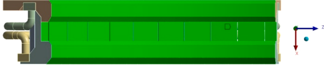
Fig. 11. The figure displays the faces of the PAS and bolometric array on which plasma thermal flux is applied, valid for both plasma scenario simulations (3.B, 3.C).
