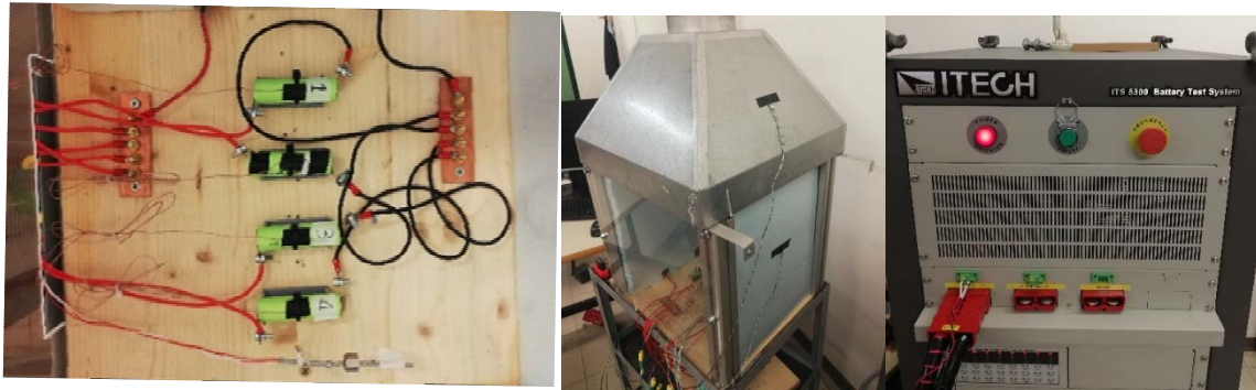
Figure 1. Test cells, complete bench and battery cycler.
