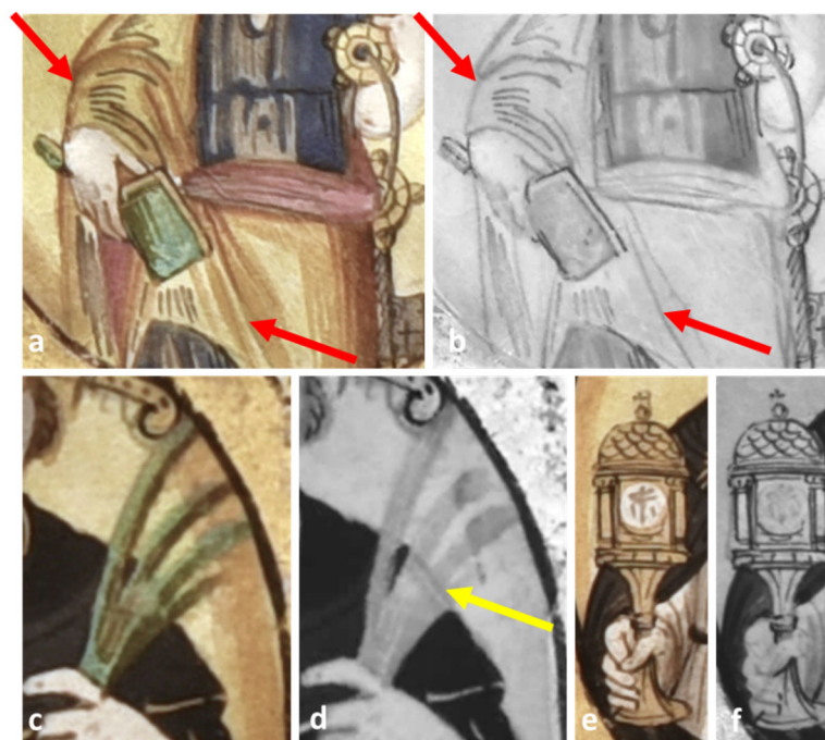
Figure 5. RGB images (a,c,e) and IRR images (b,d,f) of some details in the range 900–1700 nm (InGaAs camera). Several lines associated with the drawing are marked with yellow and red arrows.
