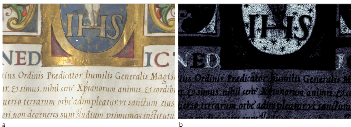
Figure 19. RGB image (a) and chromatic similarity of the blue hues. The similarity map shown in (b) is obtained by selecting the white point in the image (a). The white pixels in (b) have high chromatic similarity; the black pixels have no similarity.
