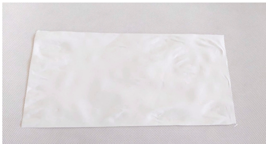
Figure 4. A sheet of polysulfone matrix membranes produced by electrospinning.
