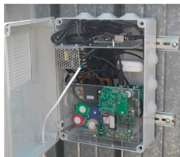
Figure 1. Sensor node AIRBOX, developed by ENEA, for urban air pollution monitoring.
