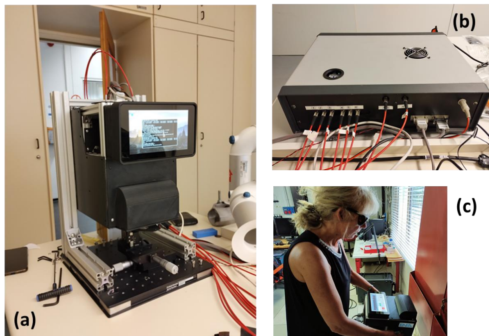
Figure 1. (a) LIBS sensor head mounted on a structure for static measurements; (b) the instrument box; (c) sensor head operated in a handheld mode.
