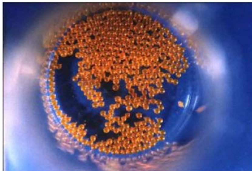
Figure 3.14.3 Fuel uranium kernel
