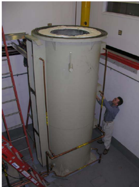
Figure 7. Production-scale CWF furnace.
