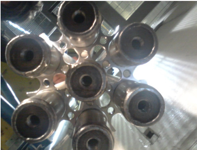
d) HERO test section, bayonet tubes ends
