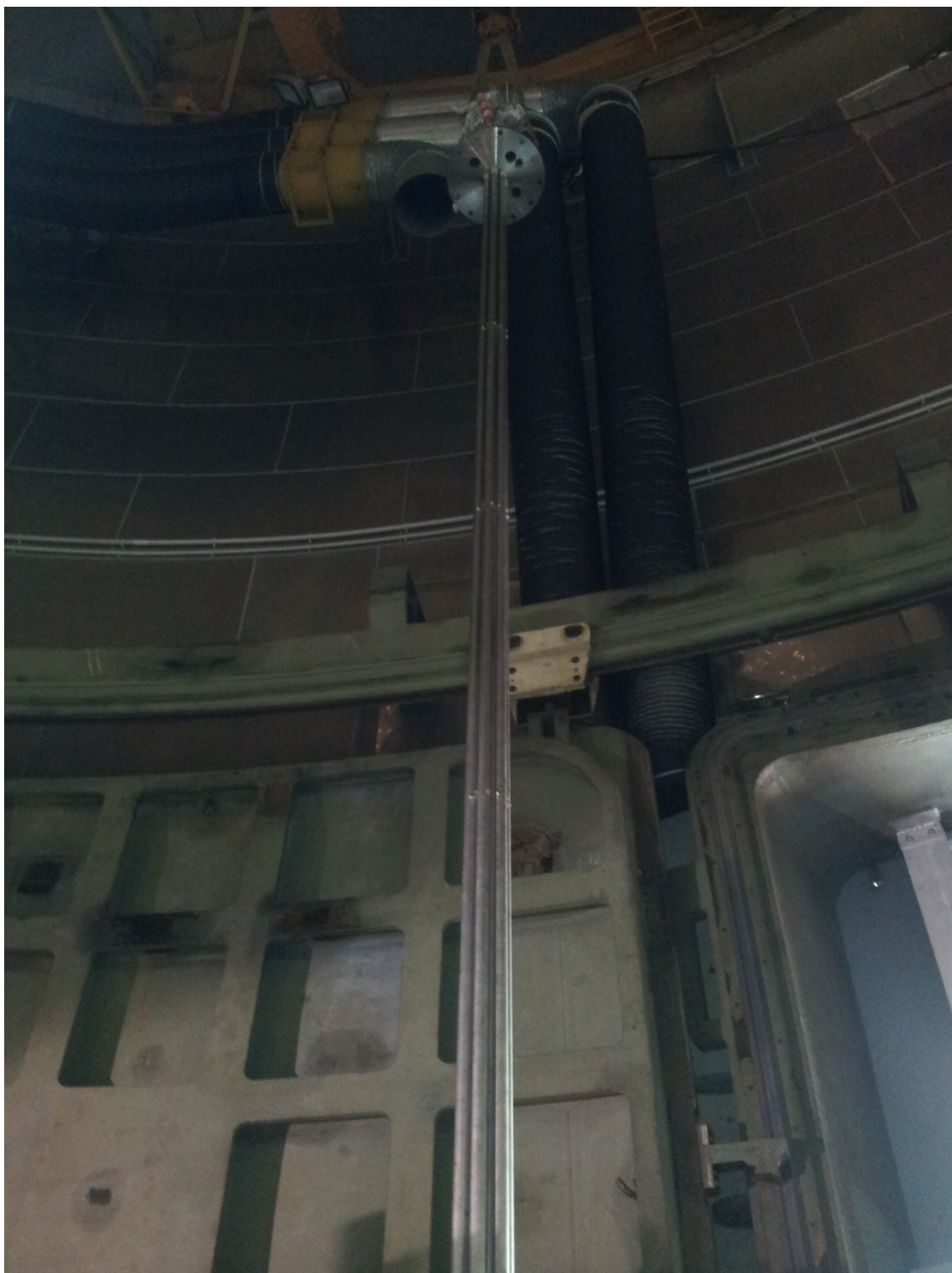
Fig. 10 – HERO-CIRCE SGBT unit: bundle arrangement.
