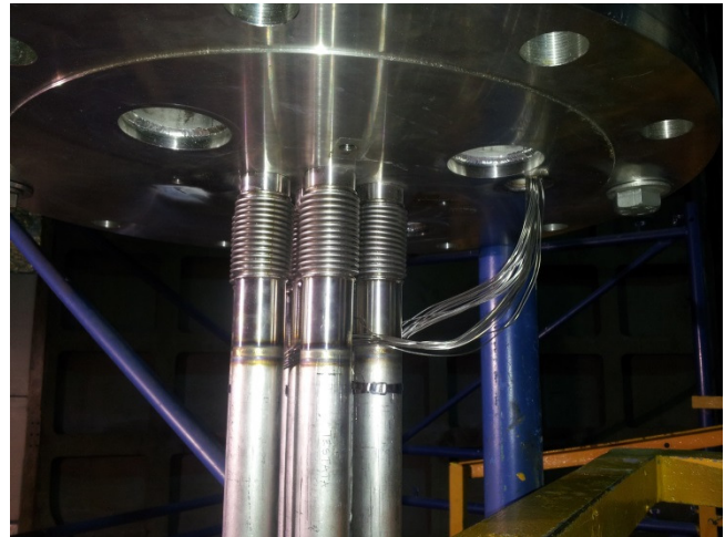
d) HERO test section, thermal compensators
