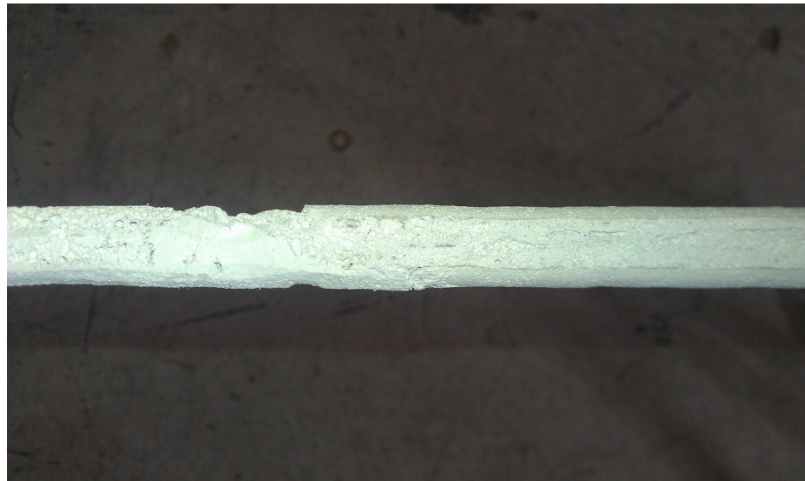
Fig. 7 – HERO-CIRCE SGBT unit, coating of ZIRCO-FOAM-250 on the slave tube outer surface.
