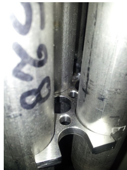
Fig. 13 – HERO-CIRCE SGBT unit: spacer grid.
