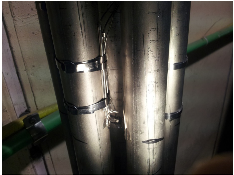
(a) TCs in the lead sub-channels
