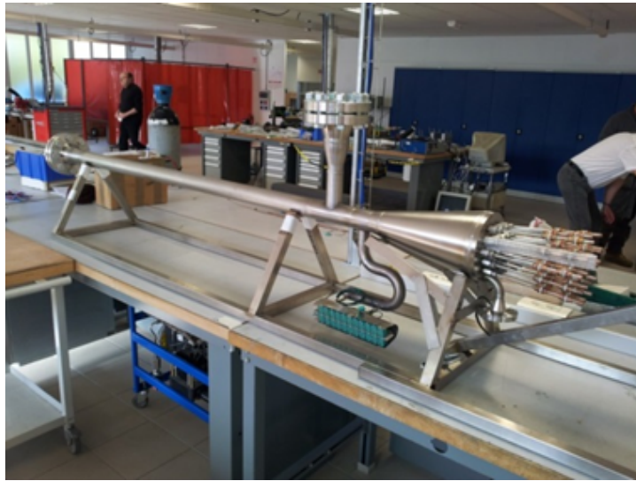
Figure.10: Fuel pin bundle simulator assembled before installation.
