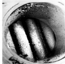
Slag deposit in heat exchanger
