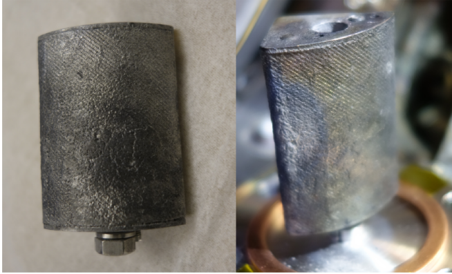
Fig. 8. Photographs of the LiSn CPS module before installation in COMPASS (left) and after the experimental campaign (right).
