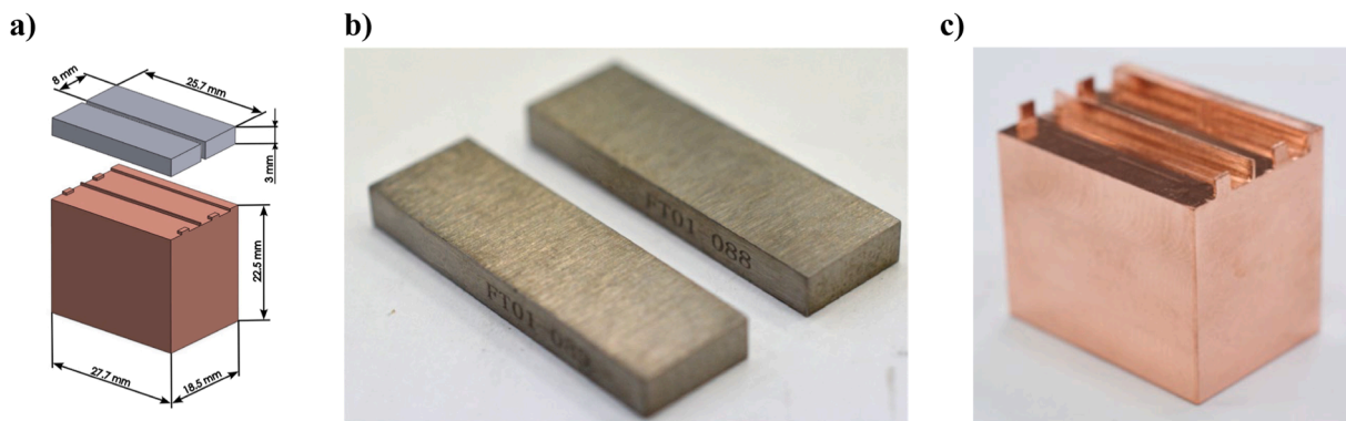
Fig. 2. Main dimensions of the W tiles and of the Cu block used for the diffusion bonding process (a); overview of some of the procured W tiles (b); Cu OFE block as manufactured from external mechanical workshop (c).
