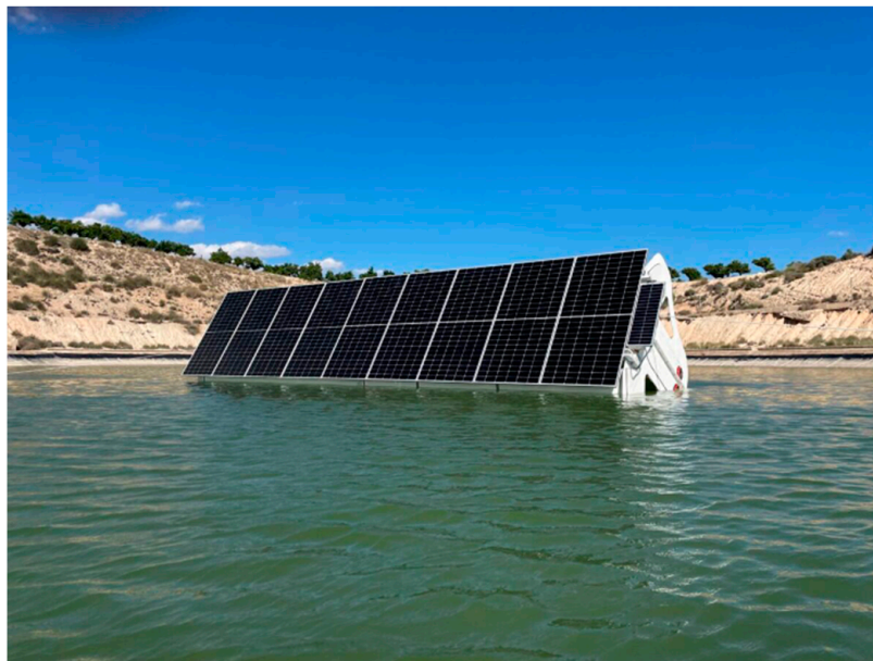
Figure 3. Photo of the experimental setup of the FLOTUS© prototype—Soltec image. Adapted from [29].
