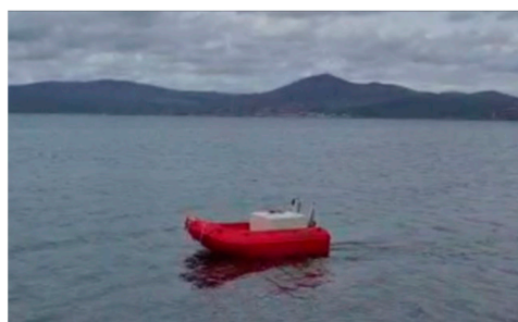
Figure 6. Two-thruster configuration during a first test on Bracciano lake.
