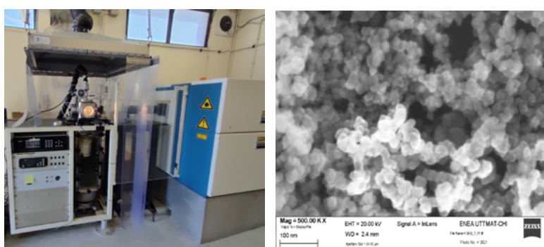
Figure 1: left: Lucifero set-up, right: SEM photo of \text{SiO}_2 nanoparticles
