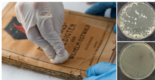
Figure 1: volume (1890) attacked by biodeteriogenes (left); growth of the microbial community before (right up) and after (right down) treatment.
