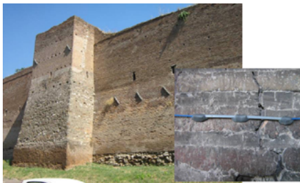
Fig 3. Pictures show a tower of the Aurelian Walls and a sensor installed on one of its cracks. The plot shows time history of one crack opening: the trend is driven by average environment temperature, with superimposed 24/h cycling due to night/day temperature variation.
