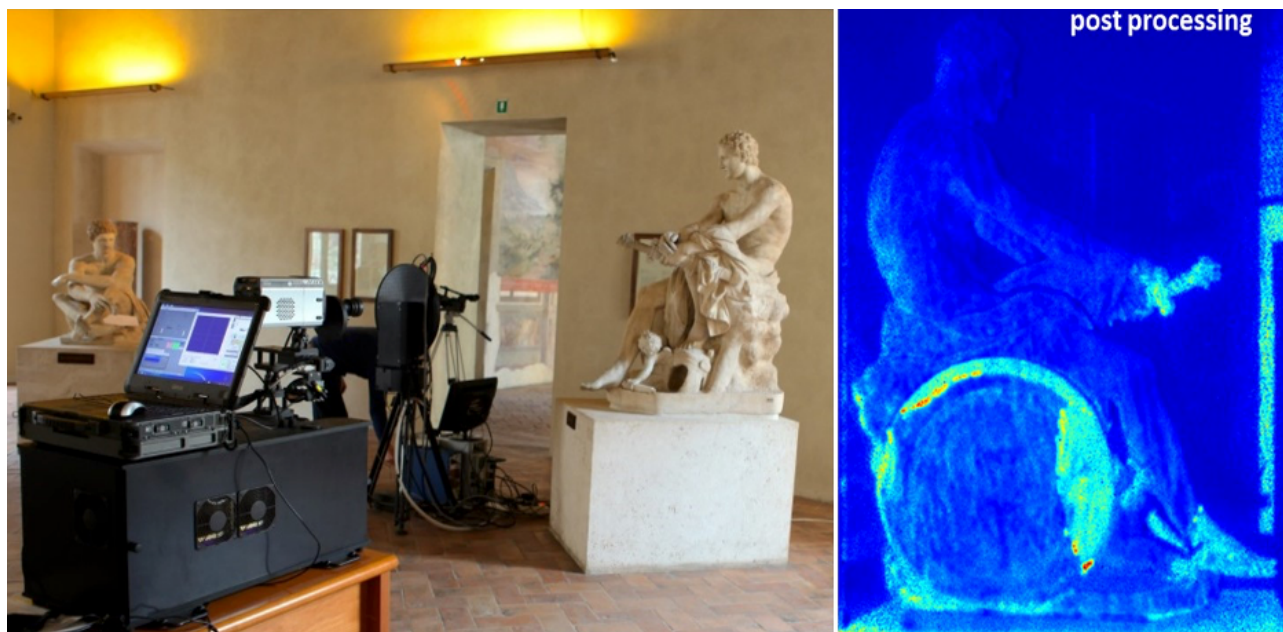
Figure 1. LIF sensors at Palazzo Altemps (left); LIF image of Ares Ludovisi after data processing (right).
