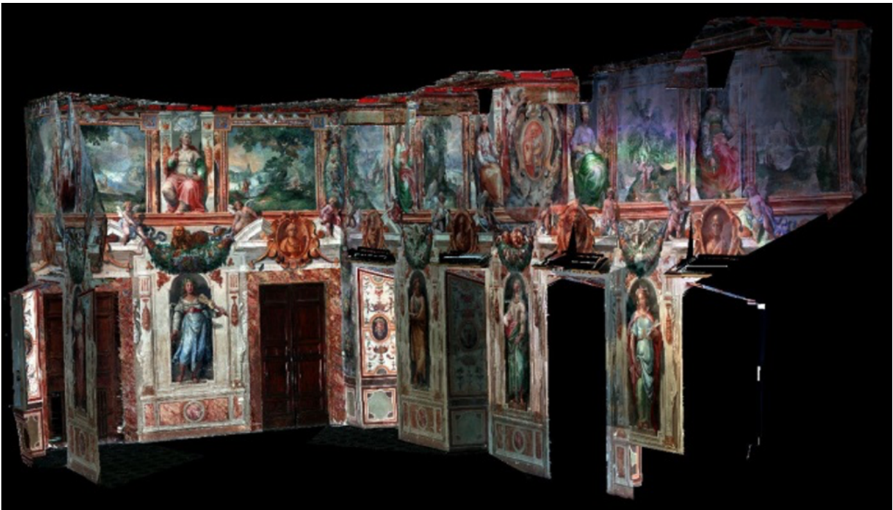
Figure 1: High-resolution 3D color model of the South Wall and of a part of the West one of the Muse Hall (Villa Sora, Frascati, Rome) obtained by RGB-ITR (ATAP project).
