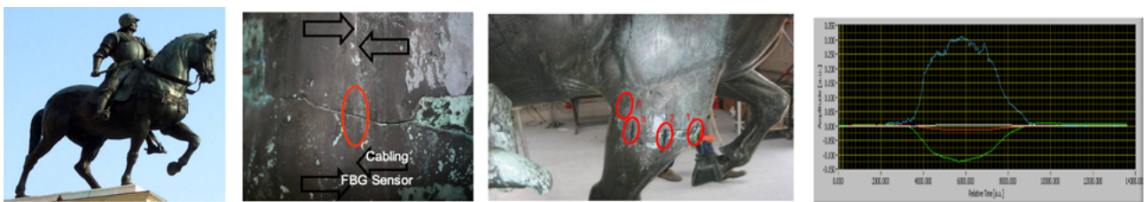
Figure 1. From left to right: the statue, particular almost invisible fiber equipped with sensor; the sensors installed on the leg; example of signals showing a transitory deformation.
