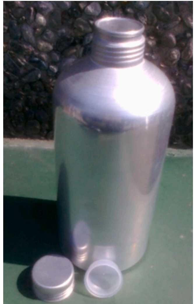
Fig. 6. Aluminum bottle containing the PCM.
