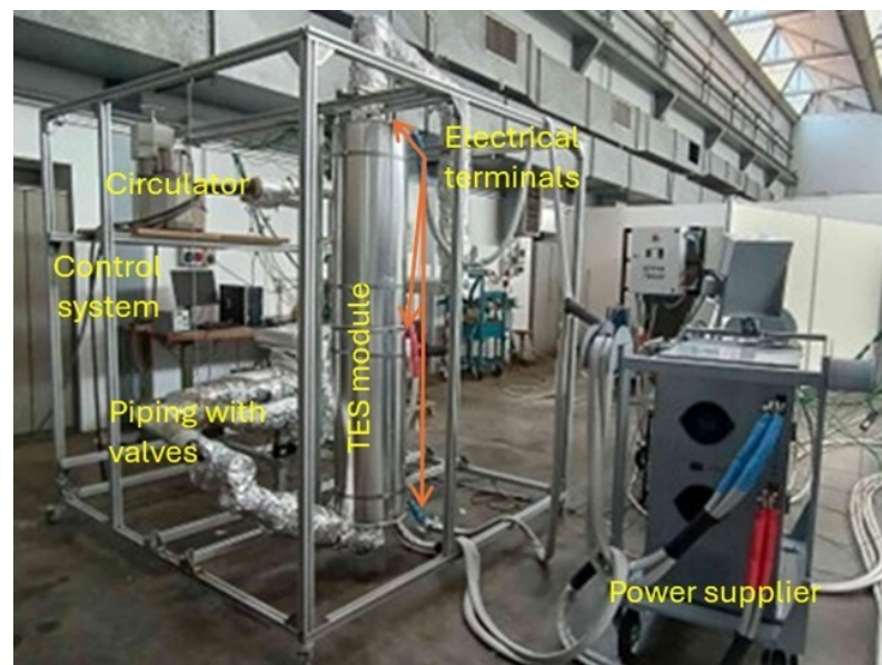
Figure 2. ATES system with the module installed and details of the power supply.
