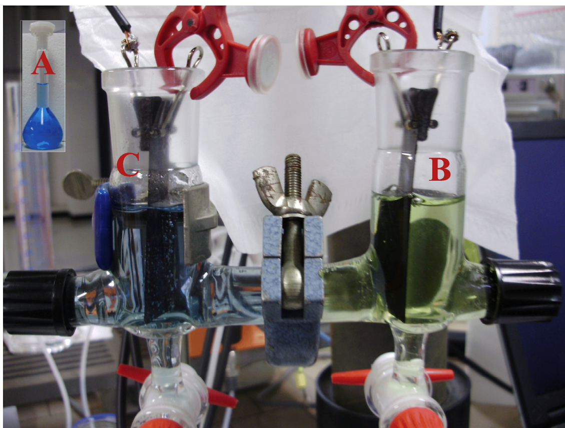
Figure 2 - Photograph of glass cell after charging step: A) initial, B) oxidised, C) reduced solution.
