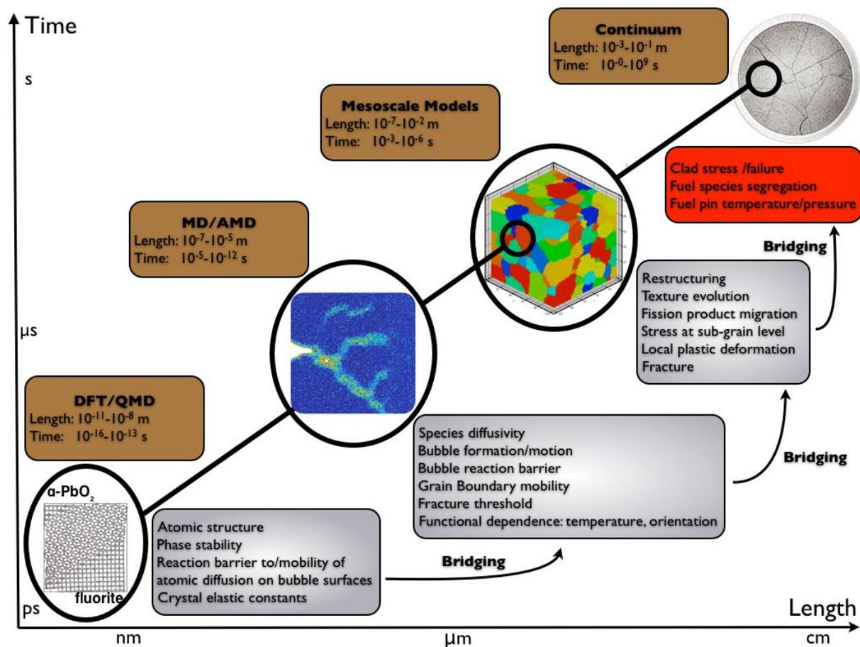
DFT: Density Functional Theory (*ab initio*); QMD: Quantum Molecular Dynamics (electronic structure); MD: Molecular Dynamics (atomistic); AMD: Accelerated MD (atomistic); Mesoscale models: grain-level techniques such as Monte Carlo, Phase Field, Mean Field; Continuum: Finite Element-like techniques.
